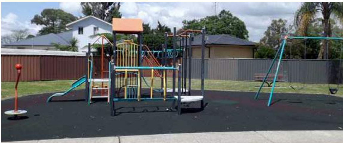
Figure 23: Unshaded rubber soft fall has been found to reach temperatures of 74 degrees on a typical summer day. Even with shade, common playground materials like soft fall and astroturf are hotter than natural groundcover (Blick, 2018).
