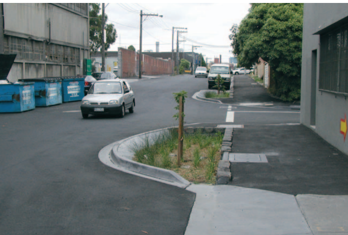
A rain garden within a verge bubble can be a useful element within any WSUD strategy depending on the design, character and topography of the street.
