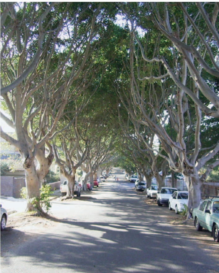
This street has the on street parking defined by both upright kerbs and street trees within the carriageway.
