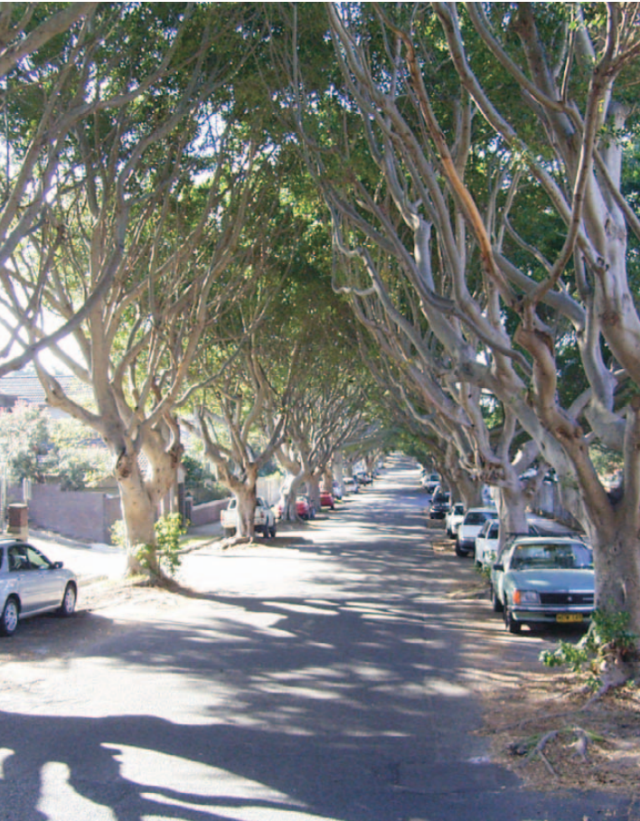
This local street has parking in bays created by trees planted within the carriageway. This street is suitable for both urban and suburban situations with its arching tree canopy.
