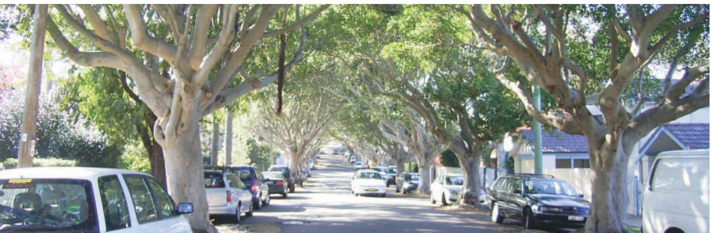
Trees within the carriageway visually narrow the width of the road whether there are parked cars or not.
