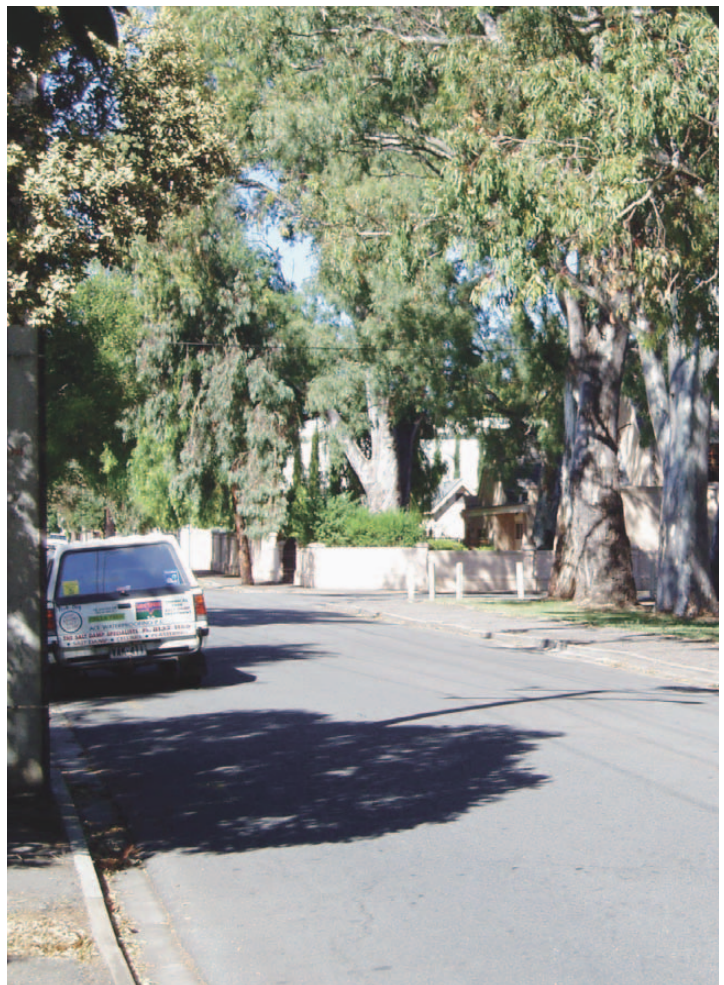
On-street parking should be provided on all streets – the design needs to respond to the type of street, number of lots accessed off the street and the character of the area. In this street the on-street parking is defined by the upright kerb as part of the carriageway with cars able to park on either side of the street.
