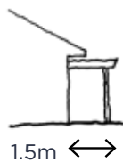
Pergola over verandah
