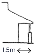
Roof over verandah
