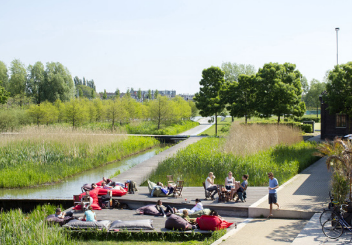
Timber walkways and terraced decks on canal adjacent to Klonneplein. Reeds filter stormwater and help maintain water quality in canal. Willow trees planted in background. Taken from (ArchDaily, 2017) Image (Thomas Schlijper)
