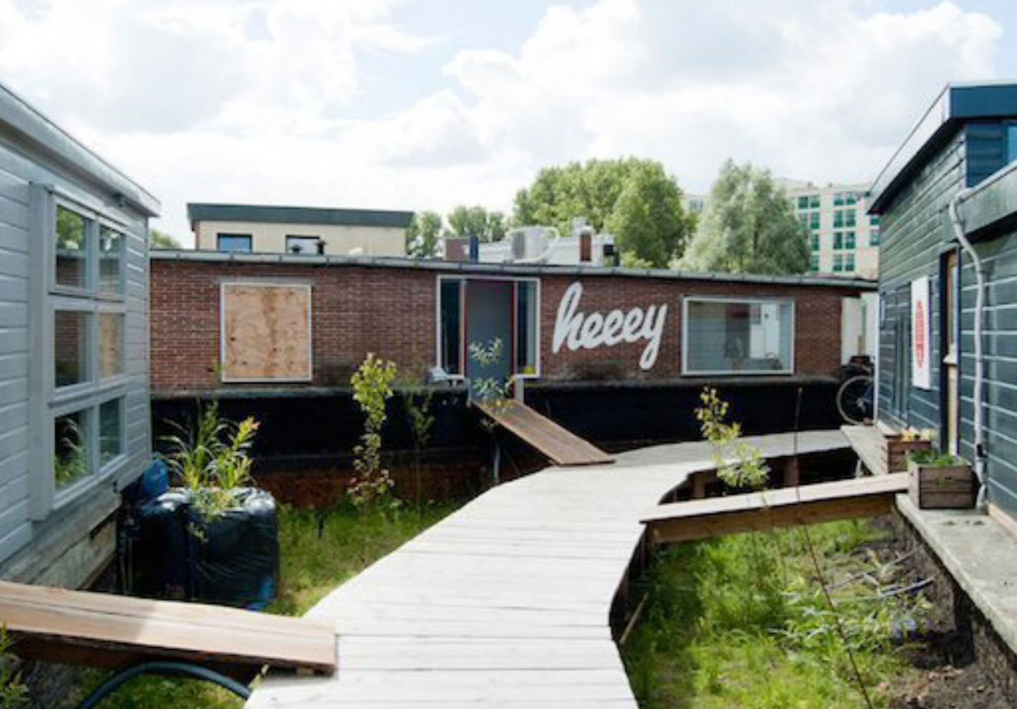
Timber winding pathway separates pedestrians from the contaminated soil and allows users to connect with the water and plants. (DEVLA Landscape Architects, 2014)
