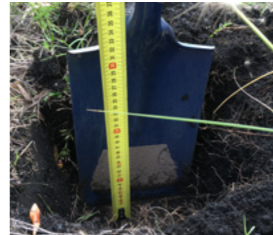
Test hole 1. Soil matrix of hummus, sandstone chips and coal dust.
